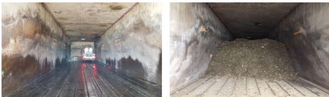
Figure 3-7 Loading of enclosed tunnels with FOGO at SOILCOs Kembla Grange facility (NSW)
